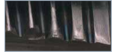
Edge chipping and wear at the chamfer.
