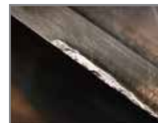
Comp. A (Severe wear, chipping)
